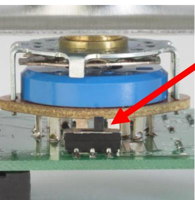
The switch on the back of the QtRC controls the lowest volume setting the knob on the front is able to produce. Depending on which direction the switch is toggled, the lowest setting on the knob is either 12 dB or completely off. This switch must be toggled prior to installation.
