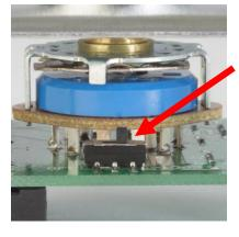
The switch on the back of the QtRC controls the lowest volume setting the knob on the front is able to produce. Depending on which direction the switch is toggled, the lowest setting on the knob is either 12 dB or completely off. This switch must be toggled prior to installation.
