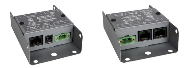
The Active Emitter Power Injector is used to combine DC power from the Active Emitter Power Supply with the audio signal from the QtPro module in order to provide a powered "signal" for the Qt® Active Emitter. There are two output ports that each support up to 25 Qt Active Emitters. The Active Emitter Power Injector can be mounted at the head end or placed in the plenum. It fits inside a standard 4x4 electrical enclosure.
