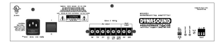
**Input:** This plug-in barrier strip provides the line-level input to the amplifier. For unbalanced input, wire high (+) and ground  $(\tau)$ . For balanced input, wire high (+), low (-), and ground  $(\tau)$ . **NOTE:** The UNBAL / BAL switch must be in the appropriate position (see below).
