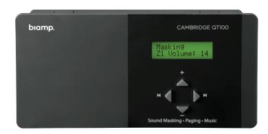
The Qt® 100 control module is a sound masking generator, controller and amplifier, with one auxiliary audio input to allow for distribution of audio from a paging controller or (background) music player. The Qt 100 control module is a compact one-zone controller suitable for installations of up to 12,000 square feet (1,115 m²). The masking level can be adjusted from the unit's front panel. Auxiliary audio level is set via the front panel.
