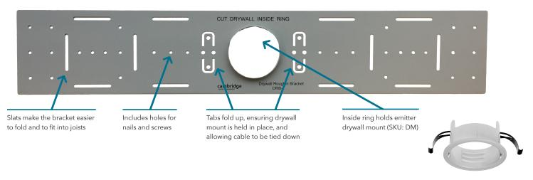
The Drywall Roughin Bracket (SKU: DRB-1) is a useful tool for installers who need to ensure that holes are left for cables and Qt® Emitters before the drywall ceiling is hung. For use with the drywall mount (SKU: DM) which holds the emitter and easily snaps into the roughin bracket.
