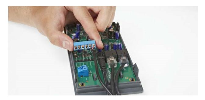
**NOTE:** The fixed terminal block can be removed for ease of connecting.
