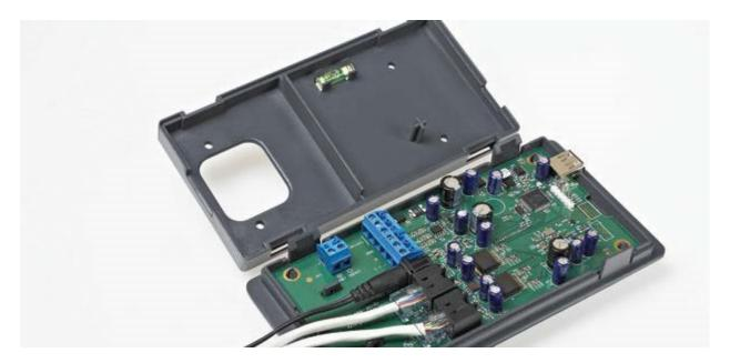
All connections are made to the control module and then the module 'snaps' into place on the wall mount.
